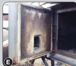
This design has several drawbacks. The outer door attempts to reduce heat loss with extremely low R-value insulation. Rubber hoses connected to the water filled inner door continually bend and can crack or fail causing damage to the furnace.
